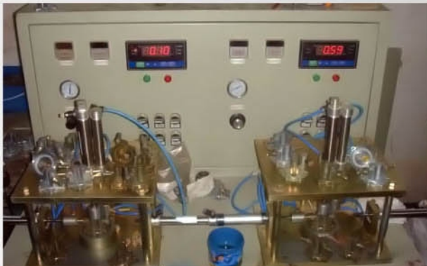
Top Housing Seal Test
